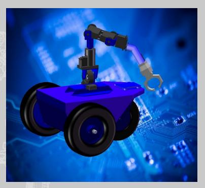
Evolution I is the first robotics configuration which is composed by 8 servomotors driven by a electronic micro-controlled board. This control board is via USB port communicated with a PC in a wired way or as an option wireless in Bluetooth protocol.
