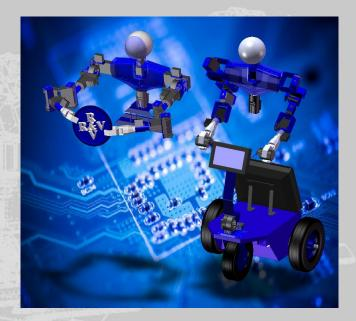
Evolution IIC is the fourth robotics configuration which is composed by 19 servomotors driven by a electronic micro-controlled board. This control board is via USB port communicated with a PC in a wired way or as an option wireless in Bluetooth protocol.
