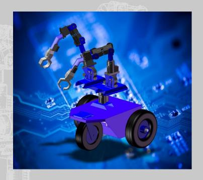
Evolution IIB is the Third robotics configuration which is composed by 17 servomotors driven by a electronic microcontrolled board. This control board is via USB port communicated with a PC in a wired way or as an option wireless in Bluetooth protocol.
