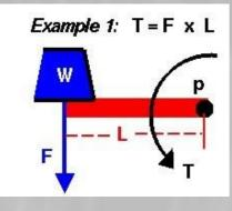
If the screw is located at point P, and is adjusted correctly when a force W of 5 Kg is applied at a distance L of one centimeter, the Torque (angular tightening force) applied will be 5 Kg-cm.
